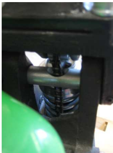
Picture.4 The correct installation of the external chain of the handle-bar is done through the hole on the cylinder.
